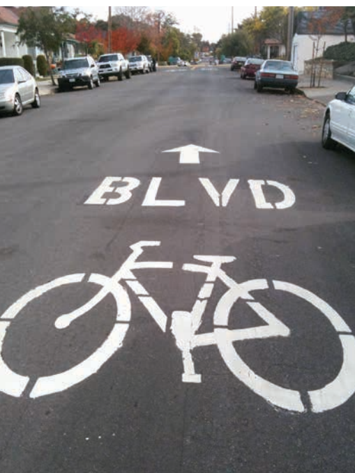
Protected bike lanes (above) provide a physical barrier between the bicycle lane and traffic and therefore a substantially more comfortable bicycling experience than conventional bike lanes. Shared roads (below) are streets in which bicycles and cars share the traffic lane.
